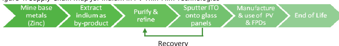
Figure 4: Supply-Chain Map for Indium in PV Thin-Film Technologies
