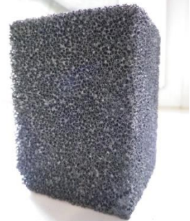
13, 20 and 30PPI \beta -SiC foams produced for simulation studies
