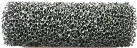
Typical 30PPI \beta -SiC foam tested in AOPs
